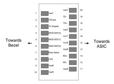
**Pinout of Connector Block on Host Board**
