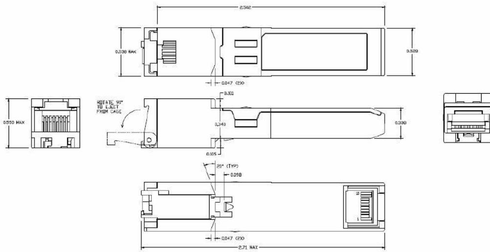
Figure 2. TOP-SFP-TF2 mechanical dimensions
