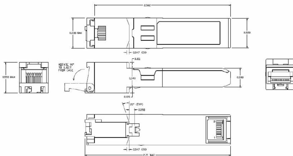
Figure 2. OLSTMRR-CNS1 mechanical dimensions
