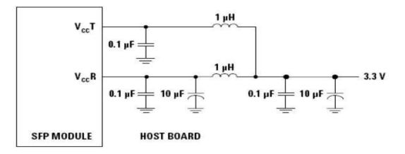
Note: Inductors with DC resistance of less than1 $\Omega$ should be used in order to maintain the required voltage at the SFP input pin with3.3V supply voltage. When there commended supply filtering network is used, hot plugging of the SFP transceiver module will result in an in rush current of no more than 30m A greater than the steady state value
