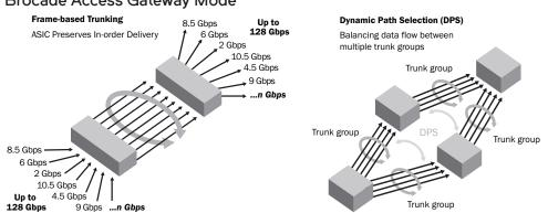
**Figure 1**: Dynamic Path Selection (DPS) augments Brocade ISL Trunking to route data efficiently between multiple trunk groups.
