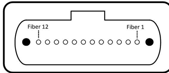
Figure 3. Outside View of the QSFP+ Module MPO
